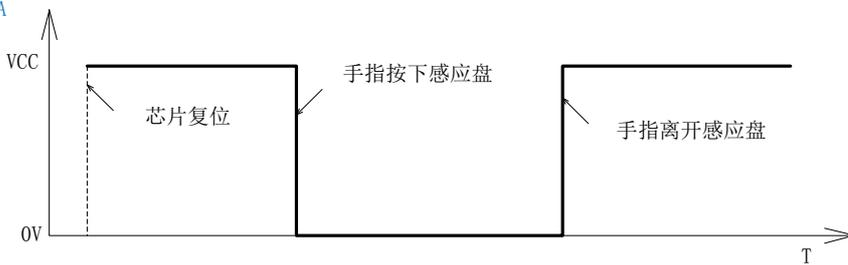
OUT电压 (外接上拉电阻)
