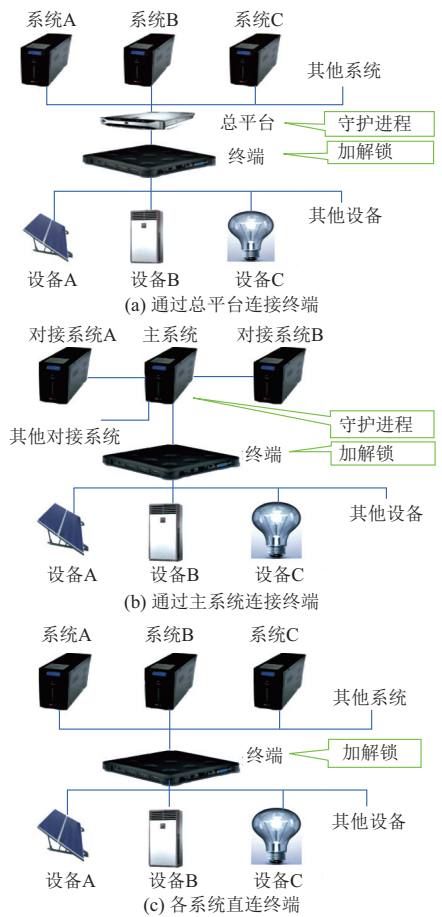
图 1 多系统与终端连接的 3 种方式 Fig.1 Three modes of connection between systems and terminals
