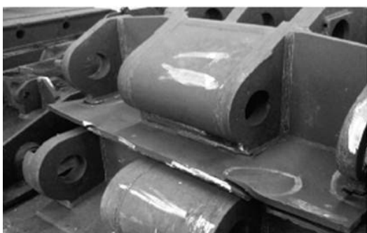
翻新前顶梁 Renovate the front beam
