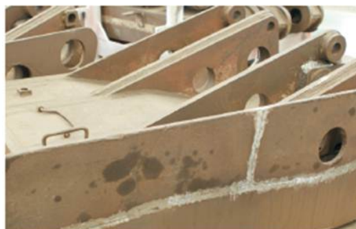
翻新后顶梁 Renovate the back beam
