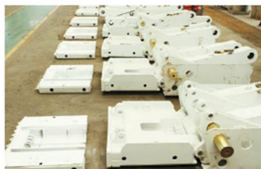
翻新后尾梁 Renovate the back tail beam
