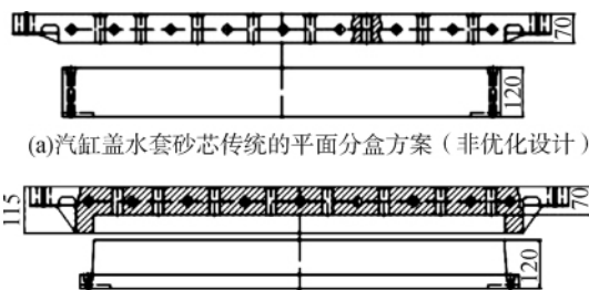
图 1 气缸盖水套砂芯热芯盒的两种不同分盒方案 Fig.1 Two different sub-box programs of hot box for water jacket sand cores of cylinder head
