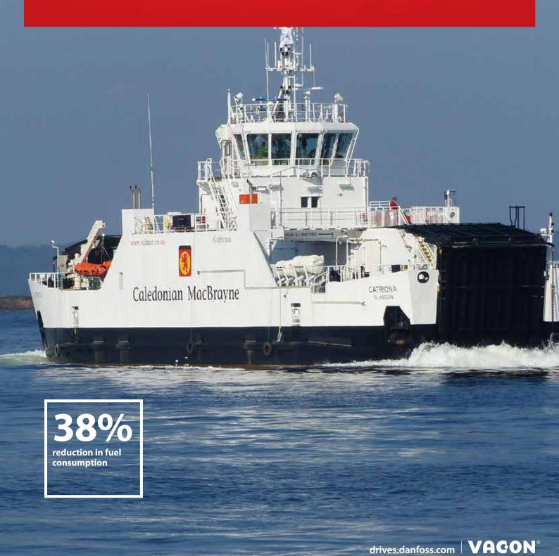
As part of its commitment to supporting Scotland's target of achieving a reduction in environmentally damaging emissions by 2020, Caledonian Maritime Assets Limited (CMAL) has developed a groundbreaking diesel-electric hybrid propulsion system for its newest roll-on/roll-off (RORO) ferries. Equipped with variable speed drives from Danfoss, this system is achieving fuel savings of up to 38% with a commensurate reduction in emissions.
