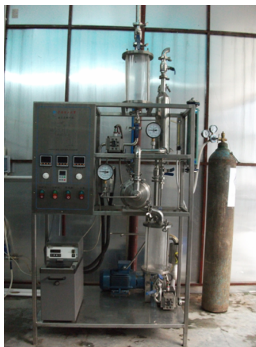
Figure 1. HIGEE-100 desulfurization equipment
