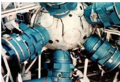
图3 NOVA laser, a 10-beam, 50,000 joule laser used for Inertial Confinement Fusion research. Look carefully to see the three technicians.
