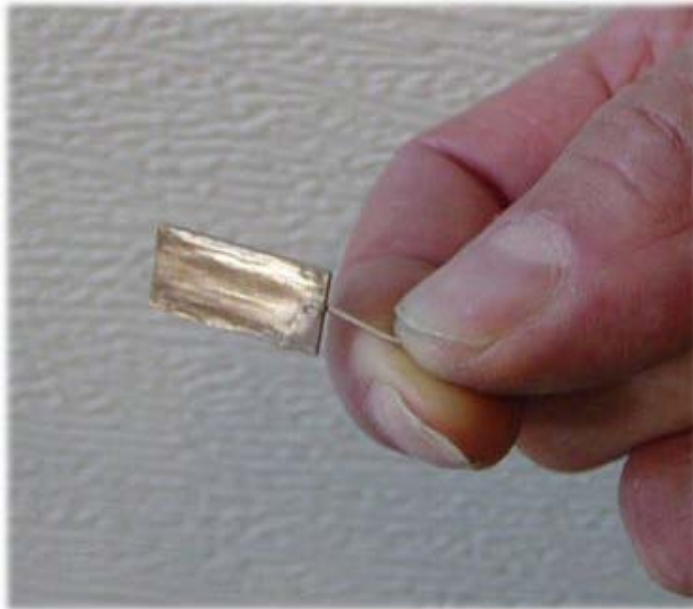
图2 Palladium Cathode used in an Electrolytic Cold Fusion Cell (Photo by Steven Krivit)
