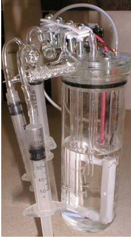
图1b Electrolytic cold fusion cell, approximately 14cm tall (Photo courtesy of Edmund Storms)
