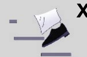
Open risers can cause fall 無踢面梯級會導致行人跌倒
