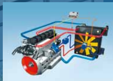
More and more “green buses” featuring Rexroth’s innovative hydraulic fan-drive system are driving on the streets of China’s cities. This system provides excellent noise reduction, and saves energy as well. 越来越多的中国绿色公交车安装了力士乐液压风扇驱动系统，从而达到降低噪音以及能耗的作用。
