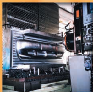
Profile Machining of an Automobile Bumper Mould Base 汽車保險桿模架加工情況
