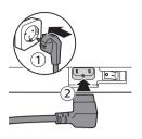
**5** Insert the power plug into a wall outlet (1) and insert the small plug into the socket located on the back of the machine (2).
