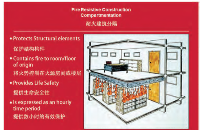
Figure 1. Example of Balanced Fire Protection – Compartmentalized Office Spaces (Source: UL LLC)
