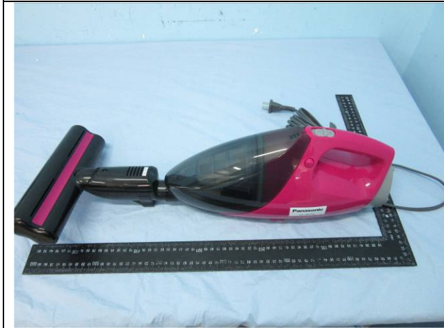
吸嘴部品编号:V96QK4 (吸嘴长250mm, 宽71mm, 管外径34mm)
