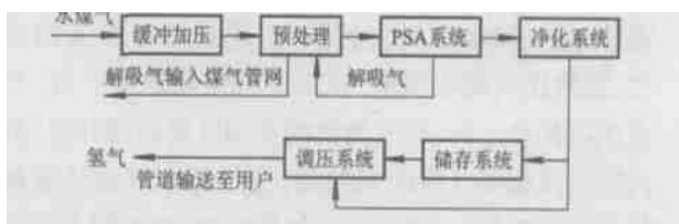
图 2 水煤气变压吸附制氢工艺流程 Fig.2 Technological process of water gas pressure swing adsorption for hydrogen
